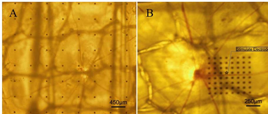
**FIGURE 1.** Two kinds of electrodes with different dimensions were used. (A) The bigger electrode array was used for field potential recording to attain global convergence of retinal neurons' signal. (B) The smaller electrode array was used for recording firing spikes and cross-correlations of RGCs to avoid the relatively coarse spatial sampling and the limited sensitivity of large electrode array. The stimulating electrode was marked.
